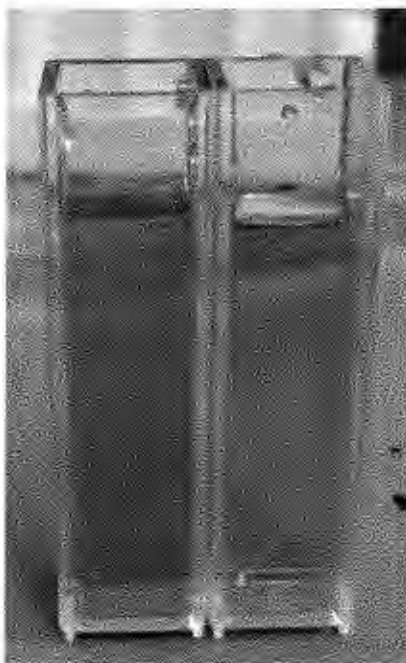
Figure 11. Comparison of silver nanoparticle solution before addition of NaCl 1.0 M solution (right) and after addition (left)
