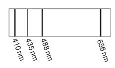
(a) Determine the energy of a photon of blue light (435nm) emitted in the hydrogen spectrum.
