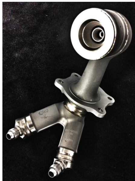
Figure 4: 3D printed fuel nozzle from LEAP engine
