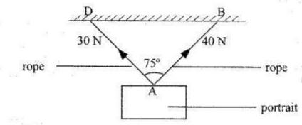
Fig. 5.11: Portrait suspended using two ropes
