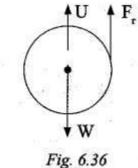
The viscous drag increases with increase in speed of the falling body.
