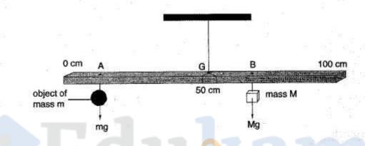
Record the distances GA and GB. Repeat the experiment by changing the position of the object or the mass M. Enter the readings of M, GA and GB in a tabular form as shown in Table 12.2.
