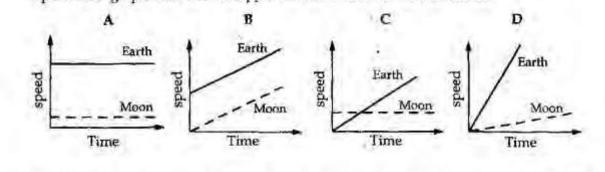
[Ans] D The gradient of the speed-time graph is the acceleration of the rock. Since the acceleration of the rock on Earth is greater, the speed-time graph of the rock on Earth is steeper compared to that on Moon.
