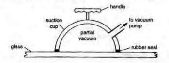
Air is removed from the cup by a vacuum pump and a partial vacuum is created inside the cup. Atmospheric pressure outside pushes the glass on to the cup.
