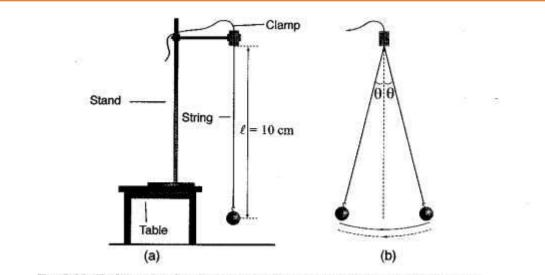
Fig. 2.28: To determine the acceleration due to gravity using a simple pendulum
