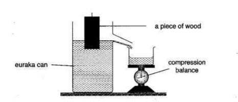
Fig. 4.1: Density of a piece of wood by displacement
