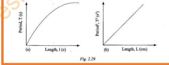
For a simple pendulum oscillating with a small amplitude, the period (T) is given bt T =  $2\pi \sqrt{\frac{l}{\pi}}$ ,
