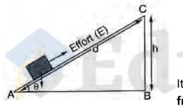
It is easier to move a heavy load from A to C than from B to C.
