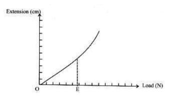
The spring undergoes elastic deformation and obeys hookes law from O to E. Beyond E, it undergoes plastic deformation hence it does not obey hookes law
