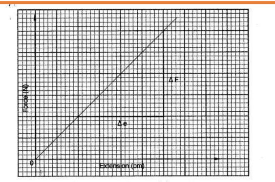
Fig. 9.2: Force-extension graph for a spring.
