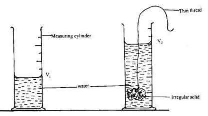
Volume of water before solid is put in =  $V_1$ Volume of water after solid is put in =  $V_2$ Volume of water displaced = Volume of Solid Volume of Solid =  $V_2 - V_1$
