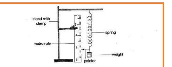
Fig. 9.1: Stretching a spring.
