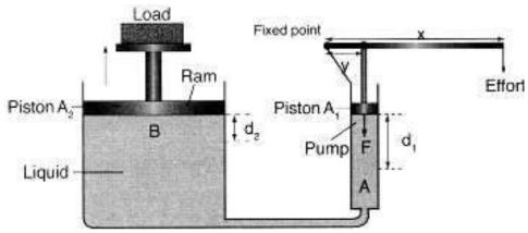
The force on the smaller piston is calculated by applying the principle of moments.
