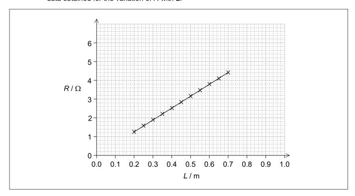
The gradient of the line of best fit is  $6.30 \,\Omega\,\text{m}^{-1}$ .
