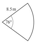
The cross-section of a gate is a sector of a circle with radius 8.5 m and angle 76°.
