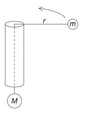
Mass *m* travels at constant speed *v* in a horizontal circle of radius *r*. What is mass *M*?
