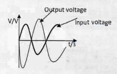
Since the transistor is a current amplifier, the amplitude of the output is greater the input: Also, the transistor is an inverter so the input and output are  $180^{\circ}$  out of phase.
