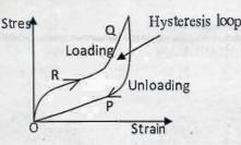
During loading, energy is supplied to the wire and released during unloading. The area under ORQ represents the work done per unit volume during the loading process. The area under the curve OPQ represents the energy per unit volume released during the unloading process. The area of the loop OPQRO represents the energy lost in the form of heat during the loading and unloading process. 2
