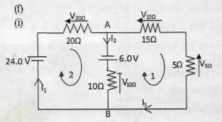
(ii)  $V_{AB} = 6.0 - 10I_2 = 6.0 - 10(0.9) = -3.0 V$ . From these calculations, it implies A is at a higher potential than B i.e the potential difference between A and B is simply 3.0 V
