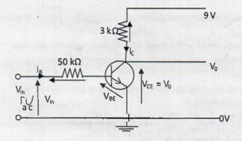
(i) Applying Kirchhoff's voltage law,  $V_{in} - I_B R_B - V_{Be} = 0 \Rightarrow I_B = \frac{V_{in} - V_{Be}}{R_B}$ , assuming the transistor is a made from silicon,  $V_{Be} = 0.6 V \Rightarrow I_B = \frac{20 - 0.6}{50 \times 10^3} \Rightarrow I_B = 2.8 \times 10^{-5} A$ (ii)  $\beta = \frac{I_c}{I_B} \Rightarrow I_C = \beta I_B = 60 \times 2.8 \times 10^{-5} = 1.68 \times 10^{-3} A$ (iii) Applying Kirchhoff's voltage law,  $V_{CE} = V_{cc} - I_C R_L = 9 - (0.00168 \times 3000) = 3.96V$
