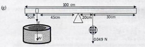
When the ring is balanced by the 5 g mass, its weight w is given by  $W(0.45) = (0.049)(0.1) \Longrightarrow W = 0.0109 N$
