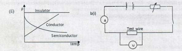
(ii)From  $V = IR \implies s \ b \ p \ e = \frac{\Delta V}{\Delta I} = R \implies R = \frac{6.4 - 2^{10}}{1.00 - 0.32} = \frac{4.4}{0.68} = 6.47 \ \Omega$  $\implies \rho = \frac{RA}{l} = \frac{\pi d^2 R}{4l} = \frac{\pi \times (5 \times 10^{-3})^2 \times 6.47}{4 \times 80 \times 10^{-2}} = 1.6 \times 10^{-4} \ \Omega m$ c)  $W = IVt = 60 \times 12 \times 60 \times 60 = 2.59 \times 10^6 \ J$
