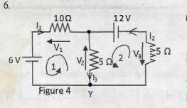
(i) Applying KVL Loop 1,  $V_2 + V_1 - 6 = 0$   $\Rightarrow 5I_3 + 10I_1 - 6 = 0 \Rightarrow 5I_3 - 10I_1 = 6 - - - (1)In$ loop 2,  $-V_3 + 12 - V_2 = 0$   $\Rightarrow -5I_2 + 12 - 5I_3 = 0 \Rightarrow I_2 + I_3 = 2.4 - - - (2)$ By KCL,  $I_1 + I_2 - I_3 = 0 - - - - - - - - - (3)$ Solving the above equations simultaneously, gives  $I_2 = I_3 = 1.2 A$ ,  $I_1 = 0$ (ii)  $V_{xy} = 5I_3 = 5 \times 1.2 = 6.0 V$
