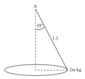
The diagram shows a particle of mass 2m kg attached to one end of a light inextensible string of length 1.3 metres. The other end of the string is attached to a fixed point A. The particle moves at a constant speed in a horizontal circle with the string inclined at an angle of  $35^{\circ}$  to the vertical.
